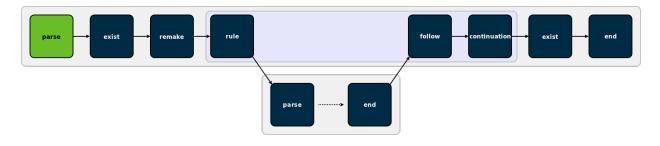
The first job in any make invocation (and therefore the first job in any eMake build) is a *parse* job, during which eMake reads and interprets the makefiles used in that make instance. The parse job's output is a list of all jobs in the make instance, along with a list of targets that must be built, the commands to build those targets, and the relationships between them.
