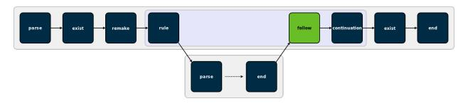
A *follow* job serves two purposes. First, it is a connection point that allows eMake to tie the end job of a recursive make invocation back into the ordered list of jobs in the parent make. Second, it is the means by which eMake propagates the error status of a recursive make to the parent make.
