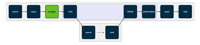
*Remake* jobs are at the center of eMake's emulation of GNU Make makefile remaking feature. In a remake job, eMake checks every makefile that was read during the parse job for two things:
