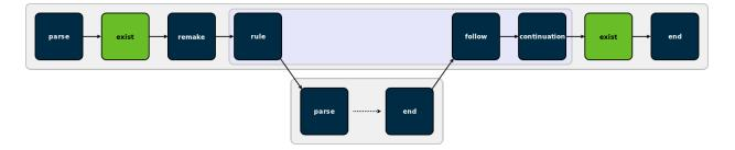
*Existence* jobs (marked as type "exist" in annotation) check for the existence of makefiles and command-line goals for which no rule was found. In the reference build, you can see an existence job in the top-level make for the makefile itself, as well as one for the file prog2, which has no rule in the makefile.
