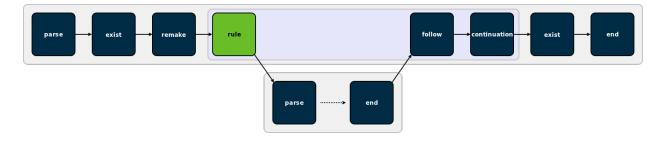
*Rule* jobs are the real workhorses of a build. Each rule job encapsulates the commands needed to update one target in the build—literally the body of a rule from a makefile—and a rule always has an associated output target (or targets), which is identified by the *name* attribute of the job tag in annotation. In the reference build, the rule job in the top-level make instance corresponds to this rule in the makefile:
