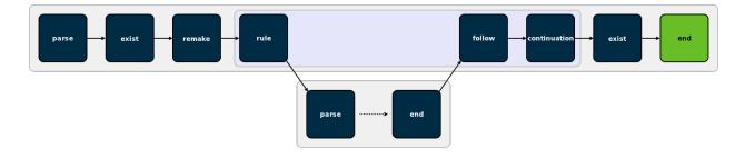
The last job in every make instance (and therefore the last job of every emake build) is an *end* job. End jobs exist primarily to handle end-of-the-make cleanup, such as removing intermediate targets or temporary inline files that were created while executing the other jobs in the make.
