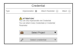
3. Select **Attach** to attach a credential to the process step. This credential is created and managed at the platform level.
