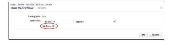
• If the parameter is checked, and after the *Build* state is completed, the workflow will immediately transition from *Test* to *Approval needed*, without starting the subworkflow.
