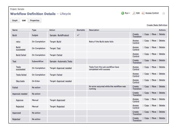
The transition order is important because transitions are evaluated in order and the first one with a condition that evaluates to 'true" is taken. In the next screen example, the *Test* state has two On Completion transitions. When the state completes, it evaluates the *Tests succeeded* transition first. If a third transition was added for the *Test* state, you could use this List view and Move the transition to the correct order for evaluation.
