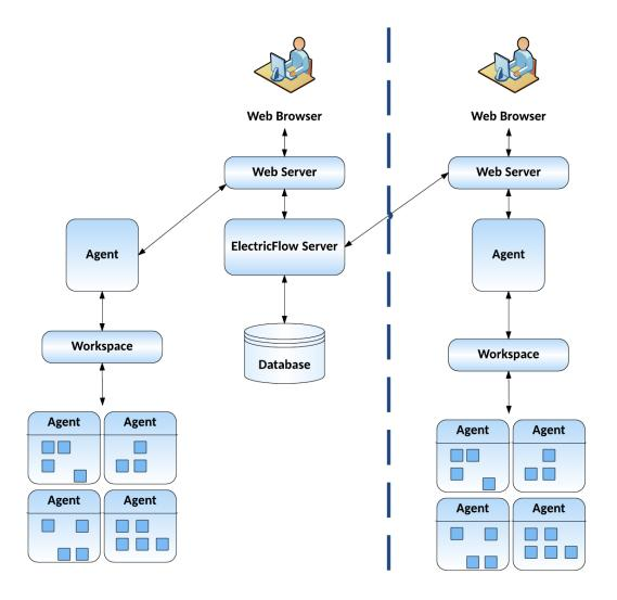
This type of remote web server configuration helps prevent network latency. If you have multiple sites, ElectricFlow can be configured to help you work more efficiently.
