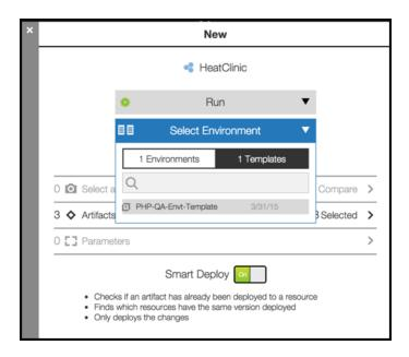
To deploy the application in a dynamic environment, you can select an environment template. A dynamic environment is created with the provisioned cloud resources. After the resources are provisioned and the dynamic environment is created, the application is deployed.
