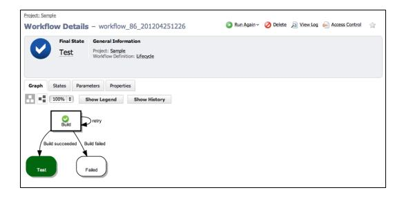
• The workflow will end up in the *Failed* state if the build fails after trying three times. (In this example, we show the Workflow History panel open.)
