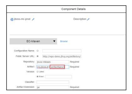
They also appear in the component process step details. When you view the component process details for the Deploy process in the Component Process Editor, you can see that the Deploy process consists of one step called Retrieve, which is defined by the jboss-mc-prod master component.
