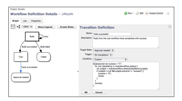
**Note:** We created the *Approval needed* state first, then we created the *Tests succeeded* transition to connect the two states.
