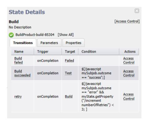
The **Parameters tab** provides a table listing all defined parameters for this state. You will see any parameters passed to this state the last time this state was entered, but only if parameters were created on the State Definitions Details panel. This table does not allow you to edit the parameter's value.
