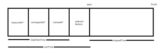
The first 4 blocks (resourceWaitTime, workspaceWaitTime, licenseWaitTime, and external factors) can occur in any order.
