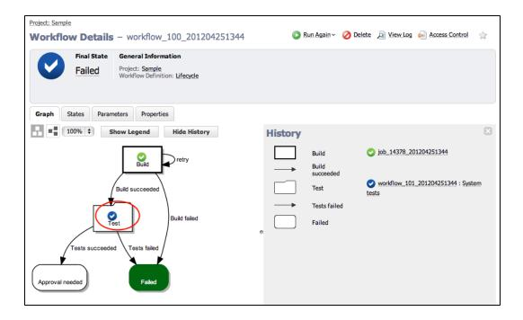
**Note:** The "blue checkmark" indicates the workflow (or subworkflow) has completed, which means it is no longer running. This icon does NOT indicate the workflow outcome (completed successfully, or with warnings or errors).
