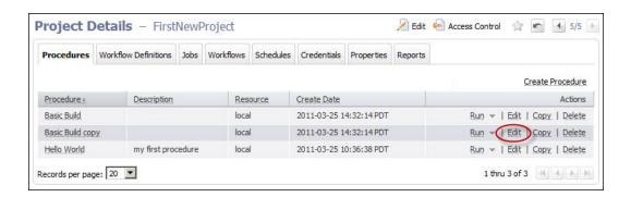
• Select the Edit link for the Basic Build copy procedure.
