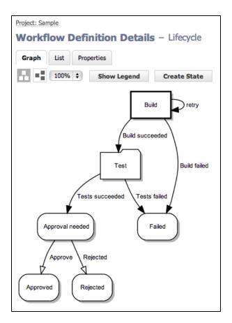
• When you run the workflow and the build and test phases succeed, the new manual transitions are made available to users on the Workflow Details page.
