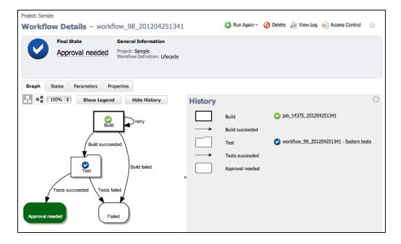
• In the following example, one of the tests in the *Test* workflow encountered an error, so the workflow will end up in the *Failed* state if either of the test jobs fail.
