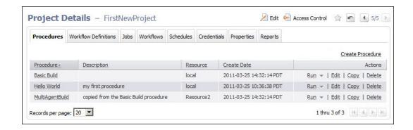
This page now displays the new MultiAgentBuild procedure with a description, and a new resource is designated for this procedure to use.
