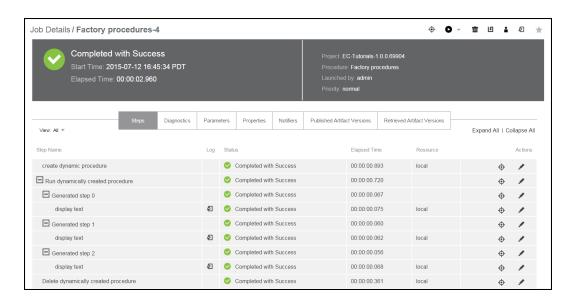
Notice the steps that execute in parallel in the dynamically created procedure: Generated step 0, Generated step 1, and Generated step 2
