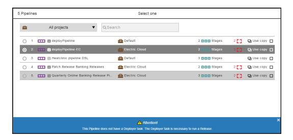
If the pipeline does not have a Deployer task, a message appears reminding you that you need to define a Deployer task to run the Release. Close the message to continue, and click **Next**.
