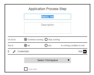
10. To define the second step in the Application Process Step dialog box based on a component, select Components > Heatclinic > Deploy. The step is defined by the component Deploy process for the Heatclinic component.
