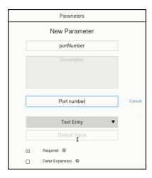
This parameter has no default value and is required. The user must enter a port number when this master component is used in an application.
