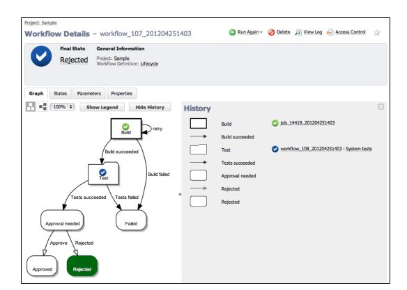
• If you choose the Reject transition, the workflow will end up in the Rejected state.
