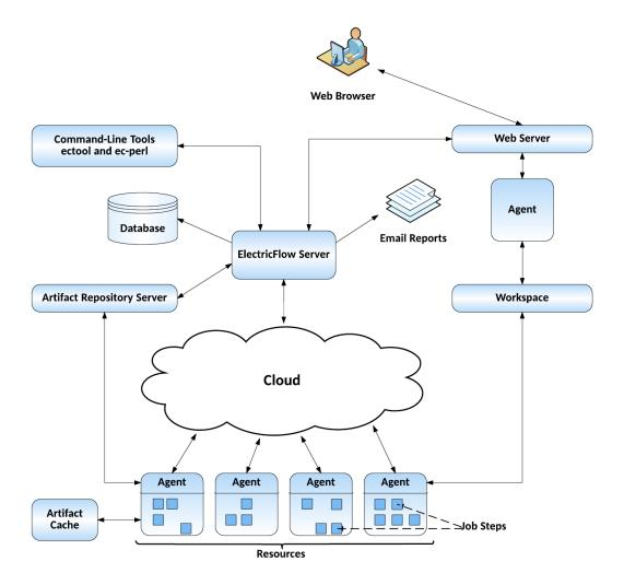
If you are only evaluating ElectricFlow, the ElectricFlow software, the database, the ElectricFlow server, the web server, and the repository server can reside on the same machine.
