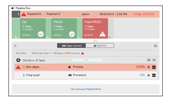
Notice that the "Run deploy" task failed and that the "Final build" task never ran because of the "Run deploy" task.
