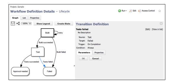
• When you run the workflow, if the test jobs succeed, the workflow will end up in the *Approval needed* state.
